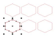
Figure 2-14 Array (X=3, Y=2)
