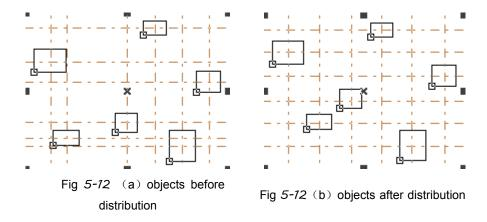
Before 'distribution' (fig 5-12a), the distance between the center of each object
