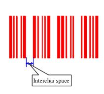
Figure 4-16 One-Dimensional Barcode Parameter Setting
