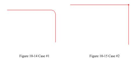
Case #2: As Figure 10-15 shows, although the right angle is what it should be, the corner of the angle is heavy marked, and this is because the Polygon TC is too long, here users need to shorten the value.
