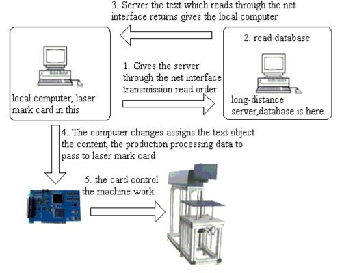
Figure 4-42: TCP/IP communication flow chart
