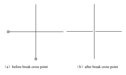
Fig 5-15 result of break cross point
