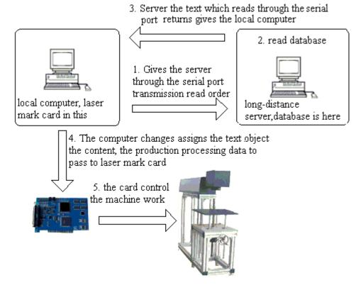
Figure 4-44 Serial communication flow chart
