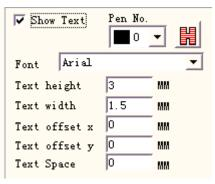
Figure 4-25 QRCODE Barcode text setting
